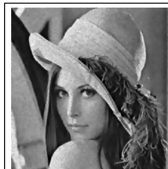
figure 2c. Reconstructed Lenna image (15-loops iterative process). Correlation Coefficient of the original image and this image is 0.9927
