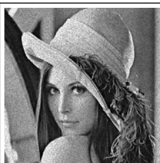
figure 2b. Noisy Lenna image (0.01-variance speckle). Correlation Coefficient of the original image and this image is 0.9836
